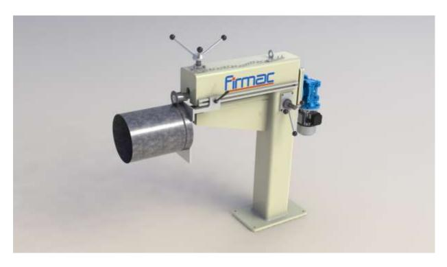
Capacities of 2mm mild steel. Operation is by foot pedal with forward and reverse control. Easily adjustable lateral movement of bottom spindle for wheel setting. (Standard electrics for 380/440 volts 3 phase 50 hertz). Low voltage. Control circuit located inside electricity interlocked cabinet with mains isolator. Supplied with one pair of standard wheels, spacing collars, lockings spanner and oil gun.
